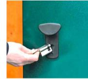
9. Carefully draw the key backwards, the barrel should slide out from the door, still attached to the key.
