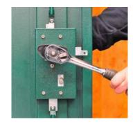
14.a. If the handle doesn't move freely you have over tightened the bolt.
