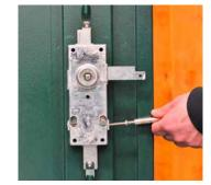
7. Remove the single pozi head screw from RH side of the side of the lock housing (this screw holds in the lock barrel)
