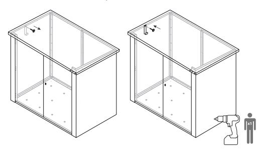
**EYELETS** (example: as installed on a Vangard shed). Select desired location for eyelet and align with nearest screw. Remove screw, and re-use to secure the eyelet to the shed.
