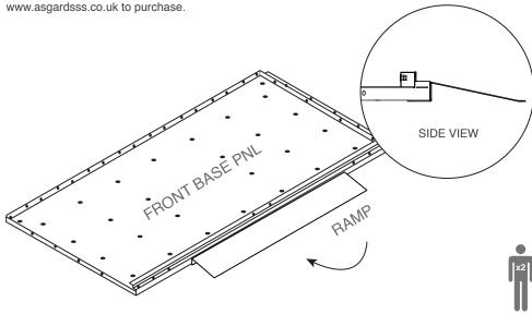
**WOODEN SUBFLOOR** (example: as installed on a Gladiator shed). All wooden subfloors are made to fit your chosen shed perfectly. Slot the subfloor on top of the each panel. These do not fix down.
