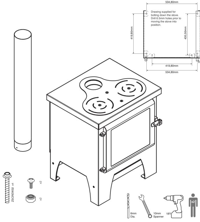
Through the into the stove and screw on the inside using 2x M4 nut & 2x screw
