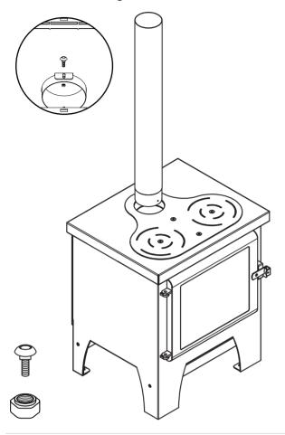
2 Drill holes in the floor using hole centre diagram (see pg1). Position your stove & bolt to floor.
