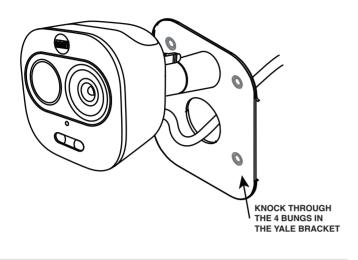
THREAD THE WIRE THROUGH THE ASGARD BRACKET AND FIX TOGETHER
