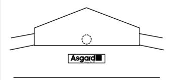
FOR OLDER SHEDS YOU WILL NEED TO DRILL A 25MM HOLE ABOVE THE ASGARD BADGE AS FAR UP AS POSSIBLE & SEAL WITH ANTI-RUST
