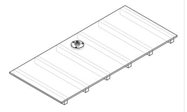
USE YALE BRACKET DISC AS TEMPLATE TO DRILL 5x M10 HOLES
