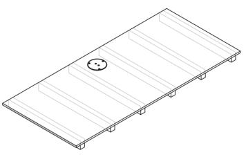
PLACE YALE ANCHOR PLATE UNDER YALE BRACKET, SLOTTING TOGETHER THE 2 CENTRE HOLES
