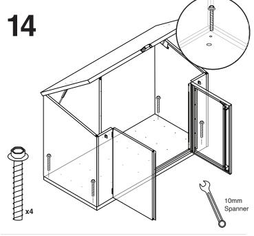
ENSURE CORRECT ALIGNMENT BEFORE ATTACHING SHROUDS (41824)
