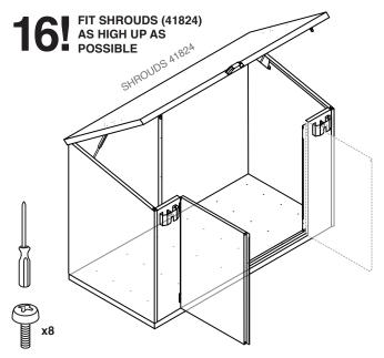
CHECK THE SHROUDS ARE FLUSH WITH THE SHED
