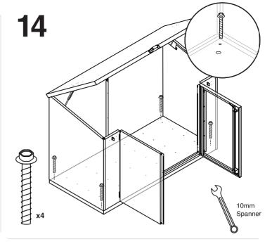
ENSURE CORRECT ALIGNMENT BEFORE ATTACHING SHROUDS (41824)
