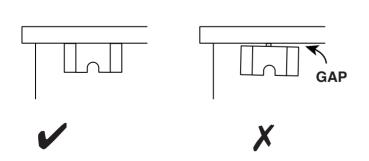
YOU MUST ENSURE YOUR BASE IS LEVEL AND THE LID ALIGNS CORRECTLY. YOU MUST BOLT DOWN THE UNIT TO KEEP IT LEVEL.
