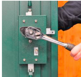
3. Remove the centre lock nut from the handle using a 17mm socket spanner (hold the outer handle whilst doing this)
