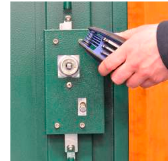
5. Using a 4mm allen key, remove the 4 bolts. Remove one pozi headed bolt from the centre of the lock cover plate.
