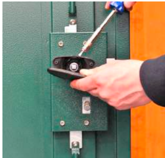
2. Remove the inner handle cover plate using a small slotted screwdriver and prise off the internal cover.
