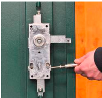
7. Remove the single pozi head screw from RH side of the side of the lock housing (this screw holds in the lock barrel)
