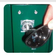
3. Remove the four allen headed bolts and one pozi headed bolt from the lock cover plate, remove the lock cover plate.
