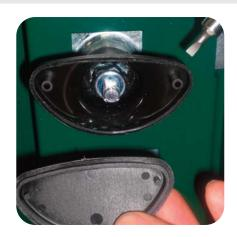
2. Remove the centre lock nut form the handle using a 17mm socket spanner (hold the outer handle whilst doing this), remove the inner handle.
